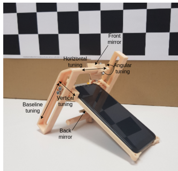
Figure A.4: The 3D printed adapter, pointing out front and back mirrors and baseline tuning. Adapted from [286].
