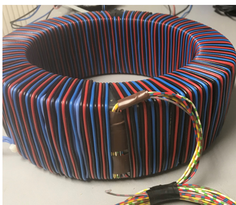
(A) Double-layered, N_e = 400 turns PVC insulated fine wire conductor
