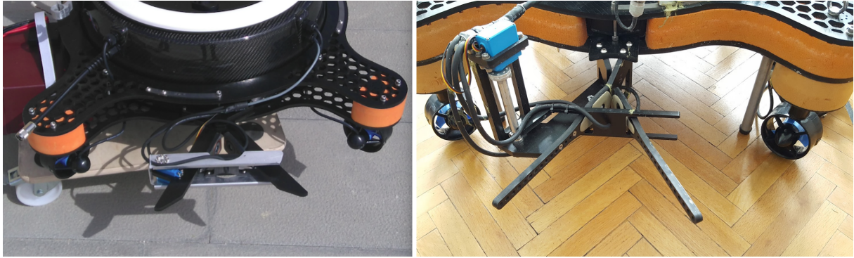
Figure 2.5: aPad-mounted docking mechanism comparison, initial design (left) and final design (right).
