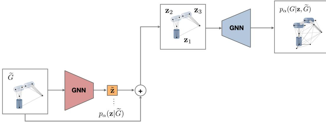
**Figure 6.3:** At test time, our GGIK solver uses the prior network  $\text{GNN}_{prior}$  (blue) to encode the partial graph into a multimodal latent distribution shown in Eq. (6.3). This distribution is then sampled and passed to the decoder  $\text{GNN}_{dec}$  that outputs a Gaussian distribution over node positions that approximates an IK solution.
