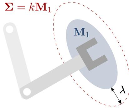
**Figure 4.6:** Singularity avoidance formulation s-IK2, in which the reference ellipsoid  $\Sigma$  produced at each iteration is a scaled variant of the original.
