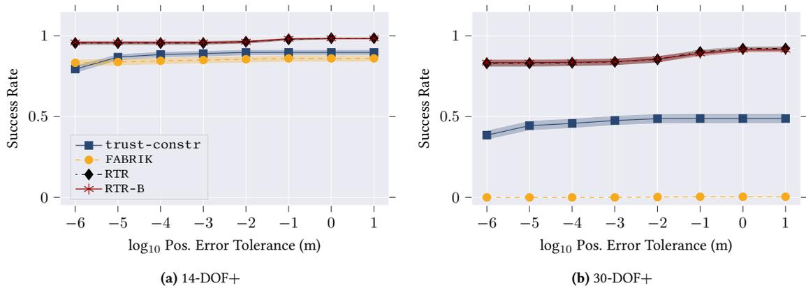
**Figure 5.7:** Waterfall curves of success rate versus position error tolerance for 1,000 experiments with planar tree robots for 1,000 experiments with planar tree robots with joint angle limits. The shaded regions are 95% Jeffreys confidence intervals centered on the solid lines. The rotation error tolerance is fixed at 0.01 rad.
