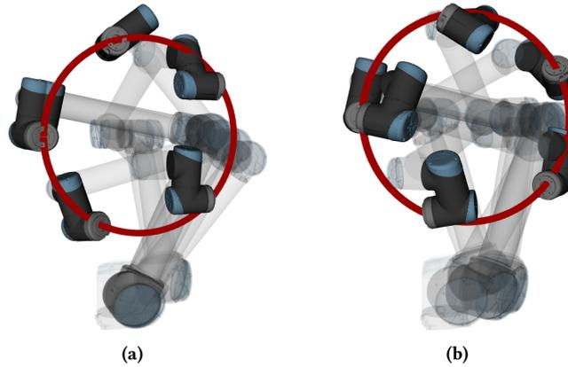
**Figure 4.9:** (a) Following a circular path with the UR10 manipulator without attempting to avoid singular configurations. Note the large change in the wrist configuration when the manipulator reaches the top of the circle. (b) Following a circular path with the UR10 manipulator while using the singularity avoidance formulation s-IK. Note that the wrist and base configurations change more slowly, improving the conditioning of the Jacobian.
