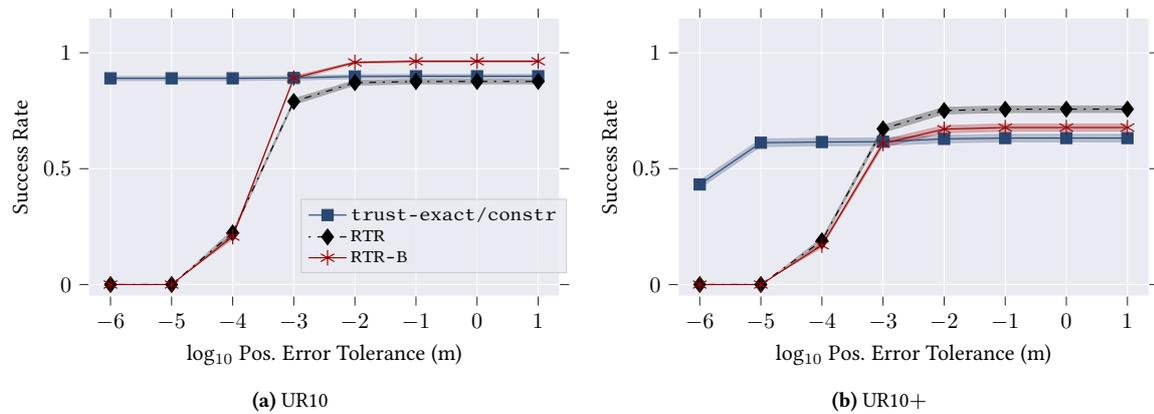
**Figure 5.12:** Waterfall curves of success rate versus position error tolerance for 2,000 experiments with the UR10 manipulator, without (a) and with (b) joint angle limits. The shaded regions are 95% Jeffreys confidence intervals centered on the solid lines. The rotation error tolerance is fixed at 0.01 rad.
