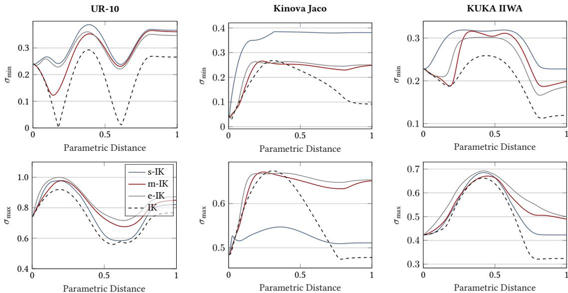
**Figure 4.10:** Jacobian conditioning throughout the circular trajectory, parameterized by  $t = [0, 1]$ . Minimal singular values  $\sigma_{\min}$  are displayed in the top row and maximal singular value  $\sigma_{\max}$  are displayed in the bottom row.
