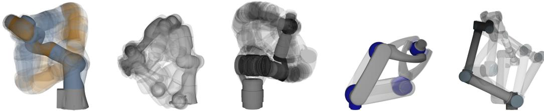
**Figure 6.4:** Sampled conditional distributions for various robotic manipulators. From left to right: KUKA IIWA, Franka Emika Panda, Schunk LWA4D, Schunk LWA4P, and Universal Robots UR10.
