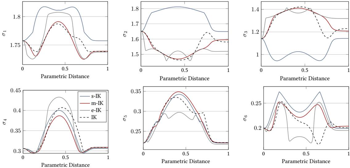
**Figure 4.12:** Jacobian conditioning throughout the execution of a circular trajectory with constant end-effector orientation for the KUKA IIWA 14 robot. The trajectory is parameterized by  $t = [0, 1]$ . Plots show how the Jacobian singular values  $\sigma_i$  change as the robot follows the path. Singular values are indexed as follows"  $\sigma_1 \geq \sigma_2 \geq \dots \geq \sigma_6$ .
