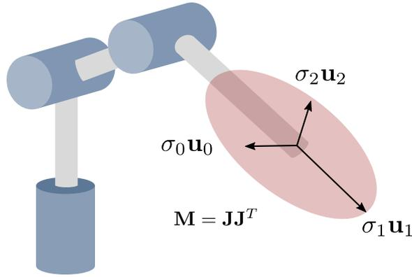
**Figure 4.1:** A three DoF manipulator and the manipulability ellipsoid associated with a task space defined by the end-effector position. Note that the axes of the ellipsoid correspond to the singular values  $\sigma$  and vectors  $\mathbf{u}$  of the Jacobian  $\mathbf{J}$ . If we were to include the end-effector orientation, the ellipsoid would be six-dimensional.
