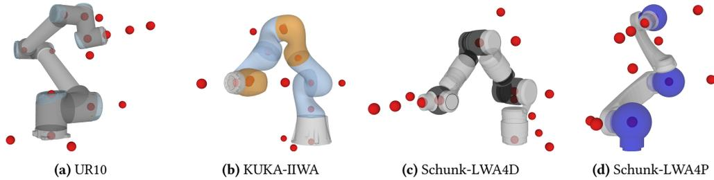
**Figure 5.10:** Points in the distance-based models of the commercial manipulators used in our experiments. Note that the distances between pairs of points on individual rotation axes have been reduced for clarity.
