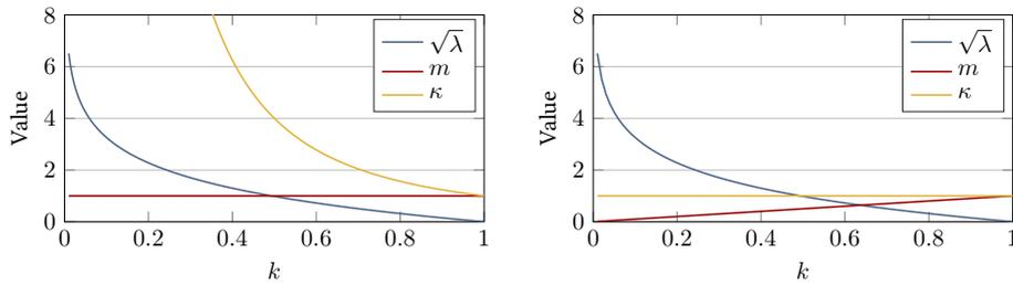
**Figure 4.5:** Performance of our geometry-aware singularity index  $\lambda$  for  $\Sigma = \text{Tr}(\mathbf{M}) \mathbf{I}$  in cases where the manipulability index  $m$  (left) and dexterity index  $\kappa$  (right) are ambiguous. The left plot corresponds to the constant volume scenario shown in Fig.4.2a, while the right plot represents the constant shape scenario from Fig.4.2b.
