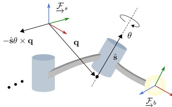
**Figure 3.2:** Sketch of the parameterization of link motions for revolute joints using screws. The vector  $\hat{s}$  is the joint's rotation axis, while  $\mathbf{q}$  is the position of some point on the rotation axis in the robot's home configuration (i.e.,  $\theta = 0$ ).
