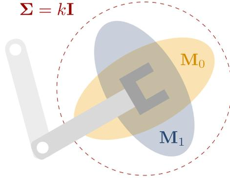
**Figure 4.4:** Singularity avoidance formulation s-IK, in which the distance between a sphere  $\Sigma = k\mathbf{I}$  and the manipulability ellipsoid  $\mathbf{M}$  is minimized. Note that both  $\mathbf{M}_0$  and  $\mathbf{M}_1$  are the same distance from  $\Sigma$ , since the squared metric  $\lambda$  is independent of orientation.
