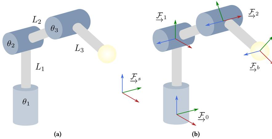
**Figure 3.1:** a) Simplified sketch of the robot structure, with links denoted by  $L$  and joints denoted by  $\theta$ . The yellow sphere represents an end-effector (such as a tool or a gripper). b) Sketch of the coordinate systems commonly defined and used in computations related to manipulation tasks.
