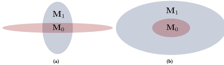
**Figure 4.2:** An example of failure modes for common singularity indices. (a) The manipulability index fails for configurations involving elongated ellipsoids with one or more axes of near zero length. (b) The dexterity index fails when the ellipsoids are of uniformly small scale.
