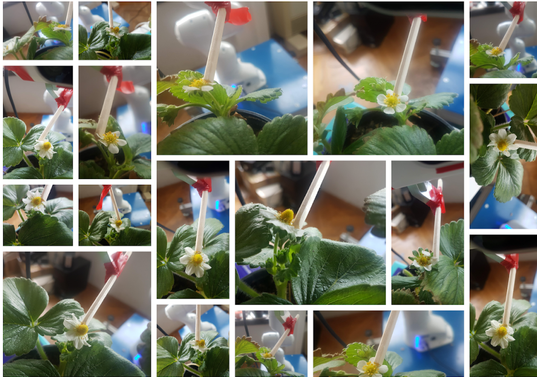
Figure 3.5: Results of the 18 successful flower manipulation experiments out of 20 trials. The example tool is positioned at the manipulation ready position, where a procedure could be executed using an actual tool.
