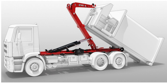
Fig. 7: Hook-loader truck example [14].
